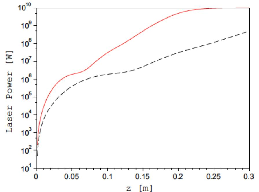
Power versus longitudinal coordinate (m) for a LPA-Wave Undulator FEL. Without (continuous line) and with (dotted line) inhomogeneous broadening effects and current density dilution due to beam transverse section increase.
