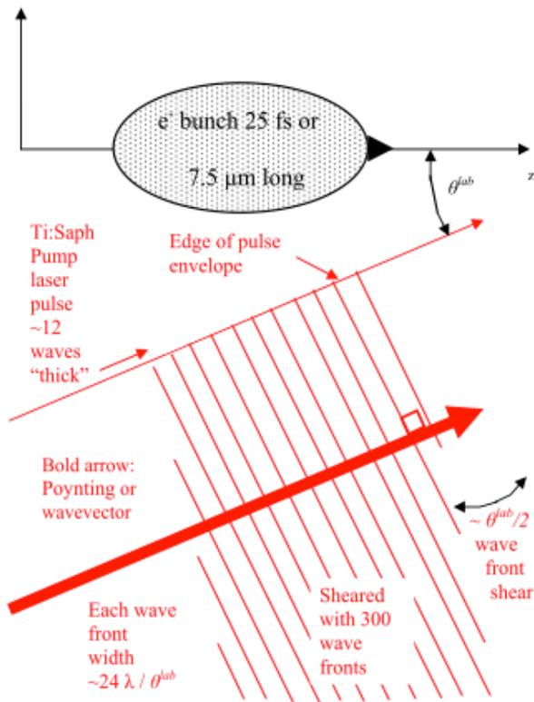
**Figure 3.** Schematic viewed from the lab frame similar to figure 2 except at an earlier time just before the sheared pump laser pulse reaches the electron bunch.
