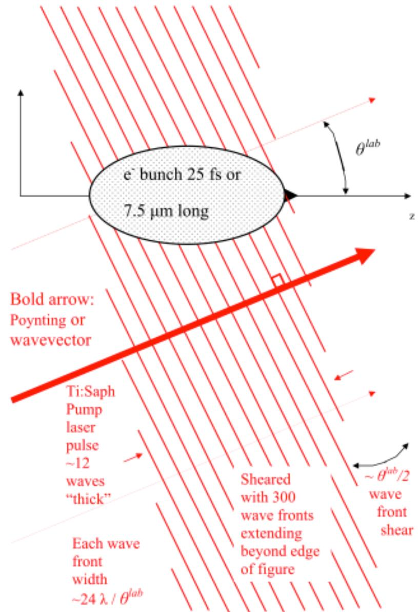
**Figure 2.** Schematic of a short (12 wave) electron bunch interacting with a sheared (300 wave) pump laser pulse ( $\lambda = \lambda_{pump}$ ) viewed from the lab frame.
