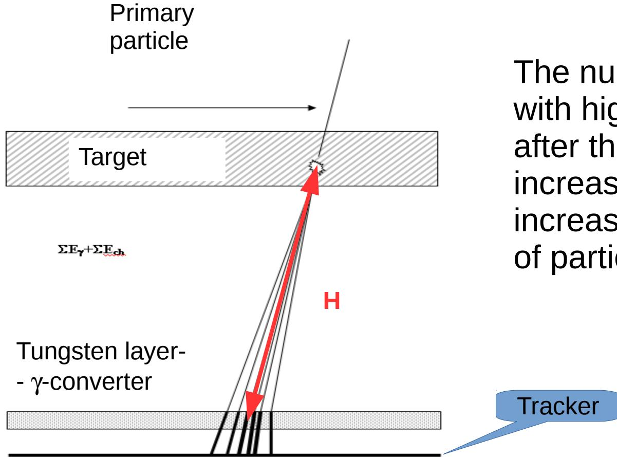
The number of secondary particles with high pseudorapidity after the first interaction increases logarithmically along increasing of the primary energy of particle
