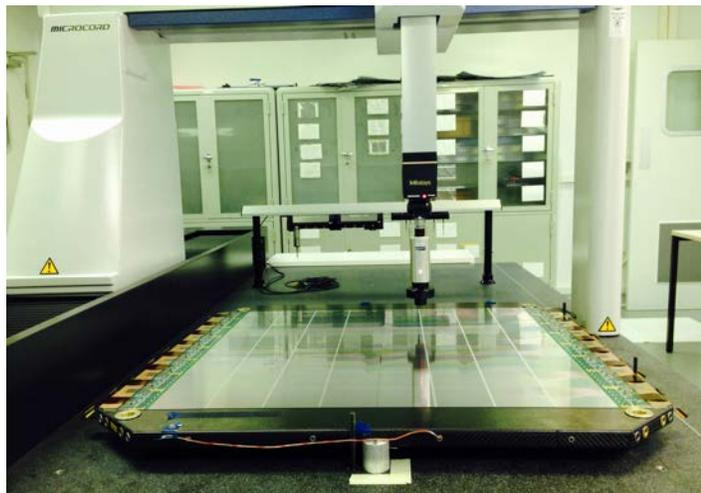
Assembled planes are measured with metrology machine, flatness  $\sim 100 \mu\text{m}$
