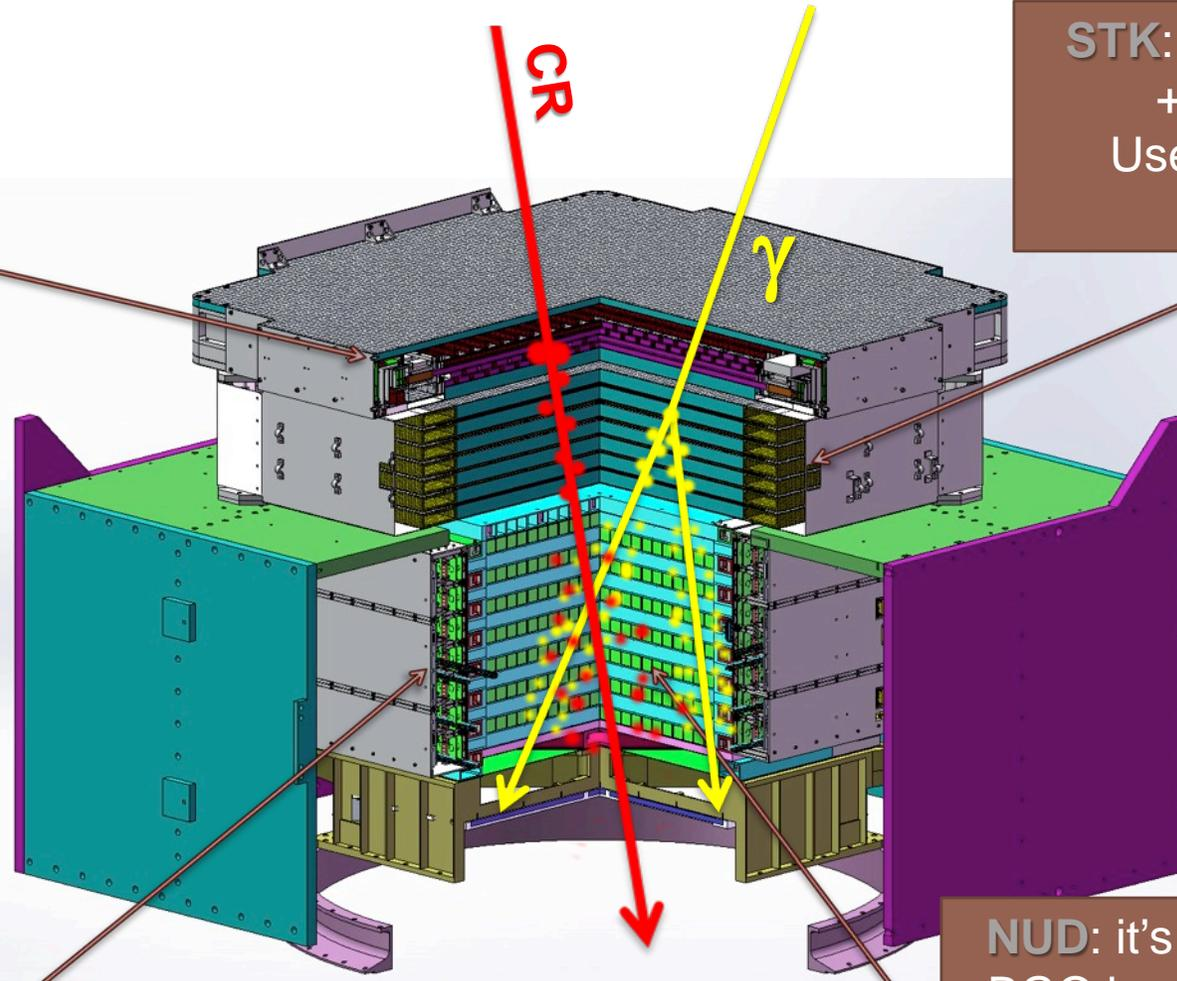
**STK:** 6 tracking double layer + 3 mm tungsten plates. Used for particle track and photon conversion
