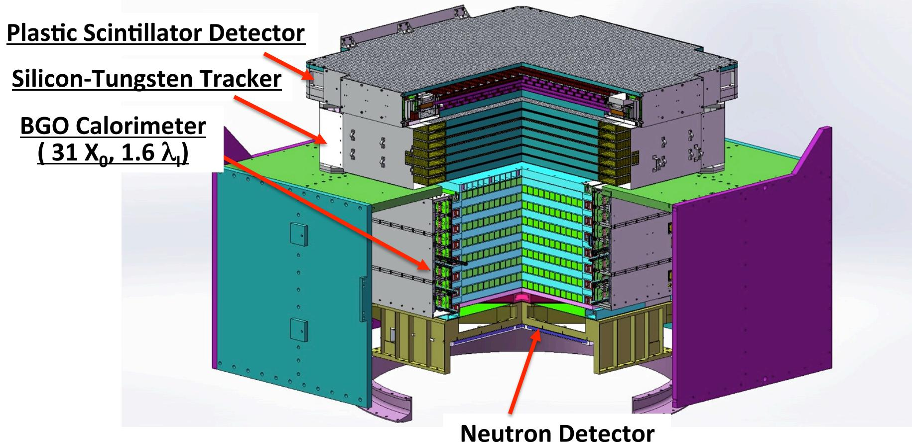
W converter + thick calorimeter (total  $33 X_0$ ) + precise tracking + chargemeasurement
