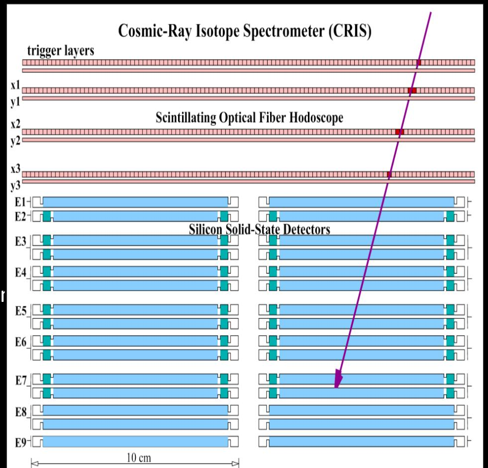
CRIS determines the charge and mass of cosmic rays stopping in a stack of silicon detectors using the  $dE/dx$  vs  $E$  technique
