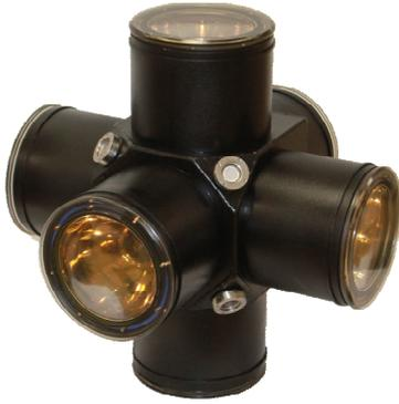
Figure 2: Quasi-spherical measuring module of the CWD NEVOD.
