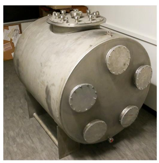
Vessel already delivered in Priceton: 1.3 m diameter 1.5 m length Made out of low radioactivity steel
