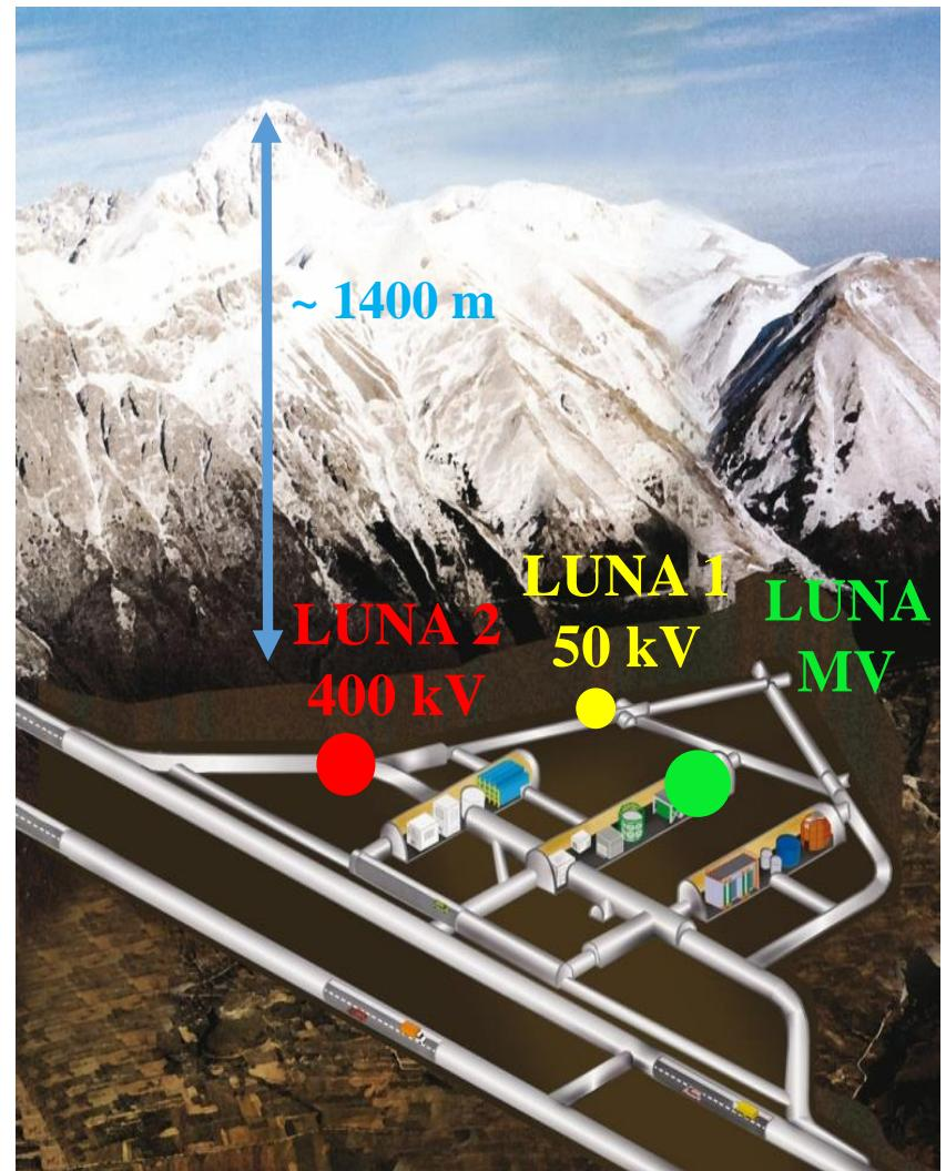
LNGS (1400 m rock shielding  $\equiv$  4000 m w.e.)
