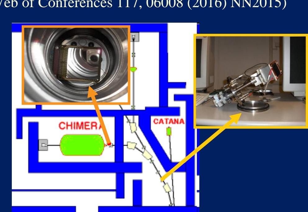
The identification of the particles is achieved by combining the energy loss in the DSSSD with the ToF information. The start of ToF is provided by the MCP. The stop is given by the signal delivered by the strips of the DSSSD.
