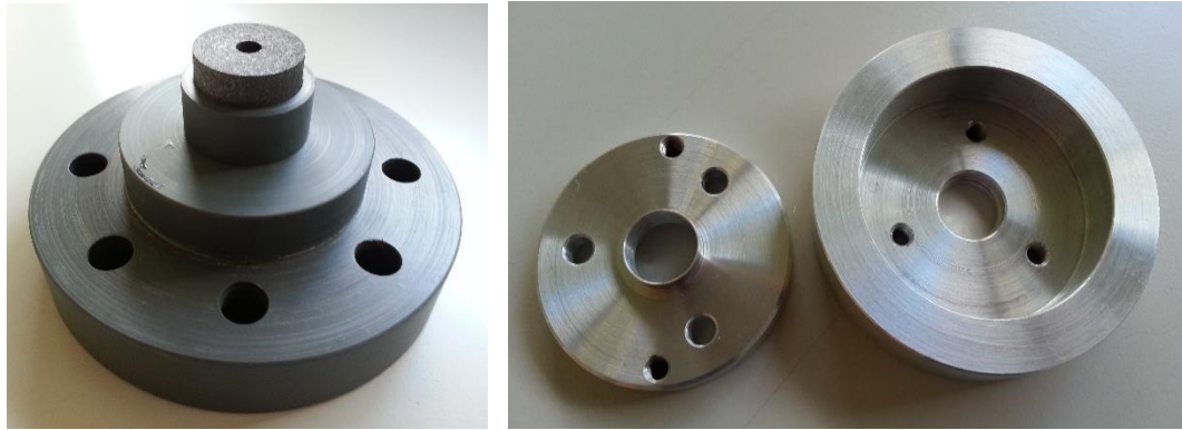
Collimator in graphite and its support (L) ; target-holder (R) Realized @ LNL
