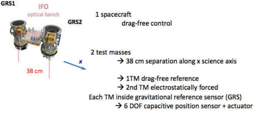
Interferometer to measure relative TM acceleration
