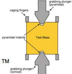
The Grabbing Positioning and Release Mechanism
