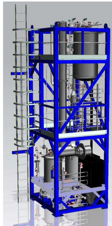
Steam stripping system
