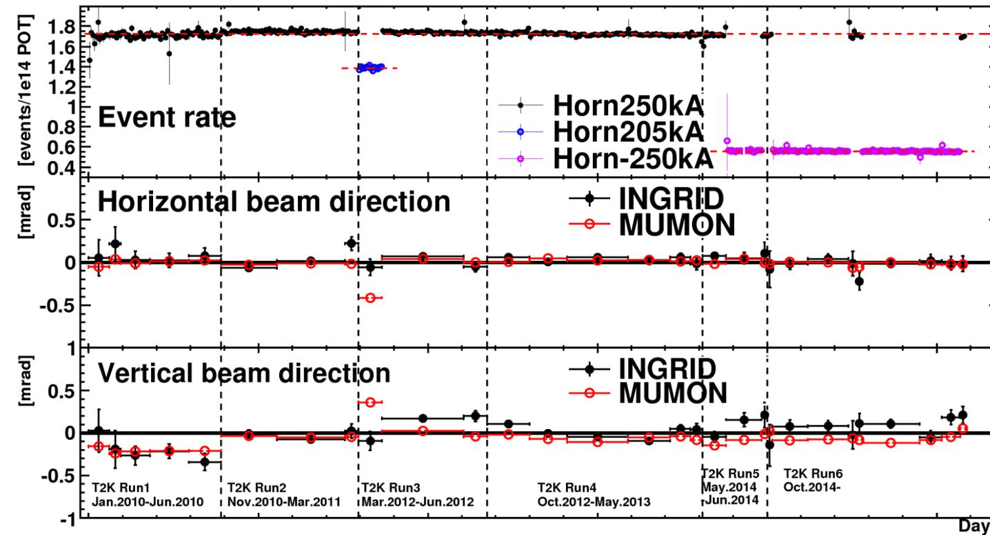
INGRID on-axis detector monitors beam stability
