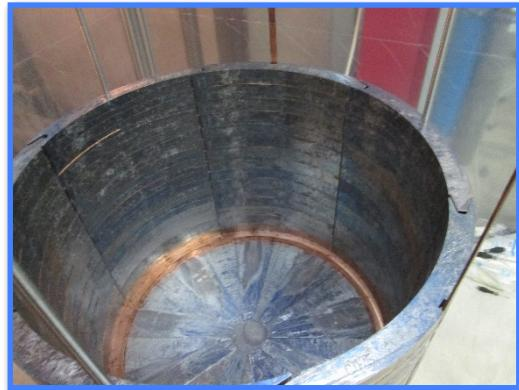
~ 5 tonnes of Pb shielding was added for Run 4. This is in addition to 2 tonnes of top Pb that was already installed previously.
