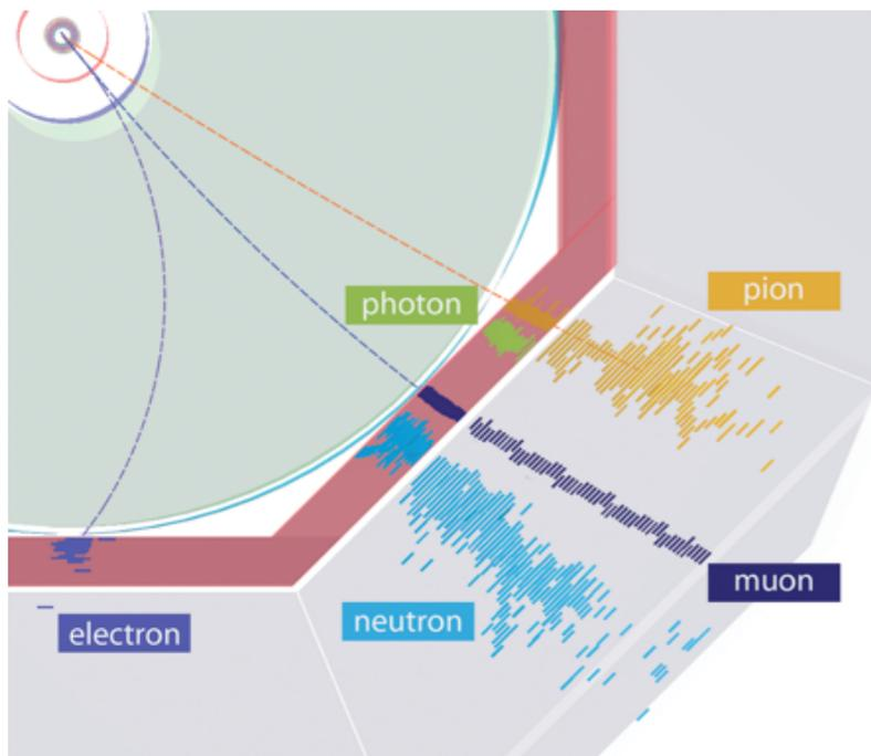
Calorimetric subsystem optimized for Particle Flow event reconstruction → high granularity
