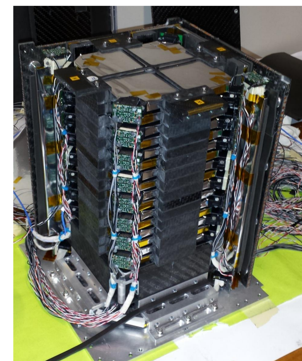
Internal of the calorimeter during the assembly
