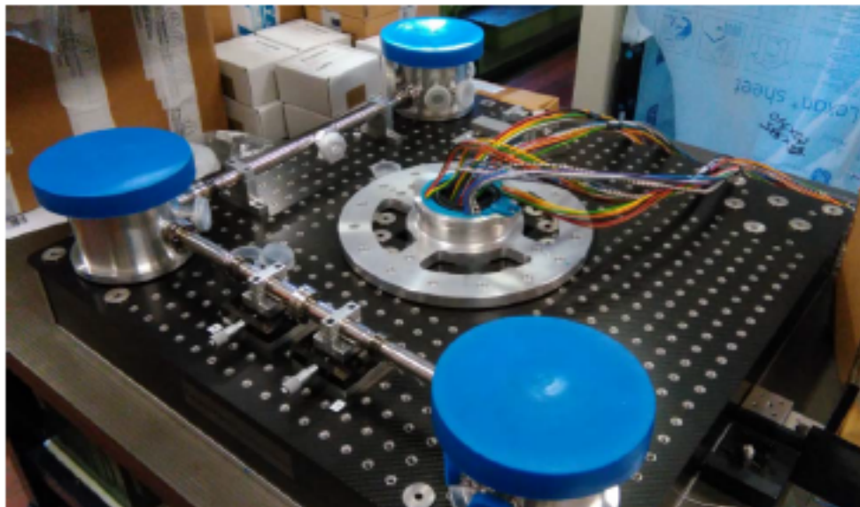
Fig. 1. Picture of the carbon fibre board mounted on the turntable. Three corner tower and two sides of the ring vacuum chamber has been already fixed on the board .
