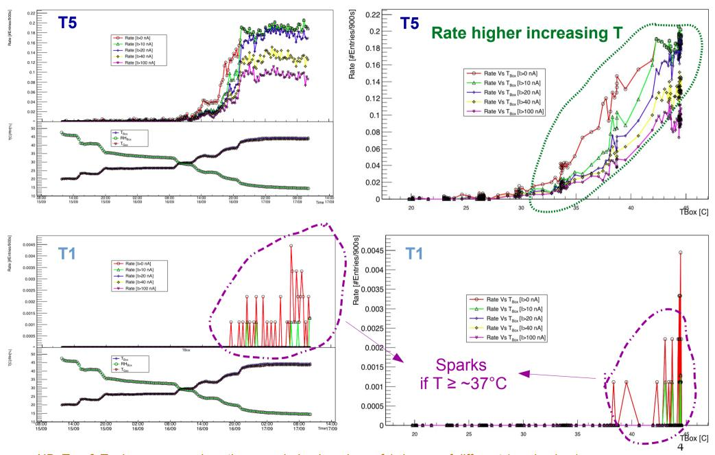
NB:  $T_{Box}$  &  $T_{gas}$  have more or less the same behaviour; less of 1 degree of different (see backup)
