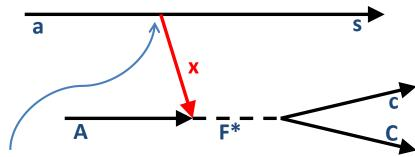
The process is a transfer to the continuum where x is the transferred particle, e.g. a proton or an alpha particle
