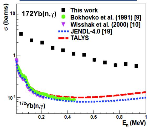
The cross sections obtained with surrogate method are in clear disagreement with ninduced data for capture!
