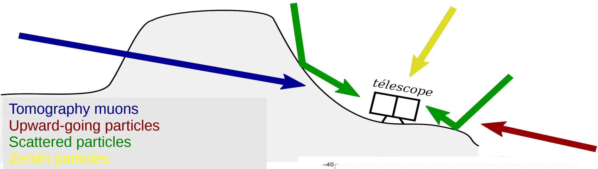
A **high precision clock TDC** technique allows a TOF analysis to disentangle particles coming either from **the front or the rear** of the telescope
