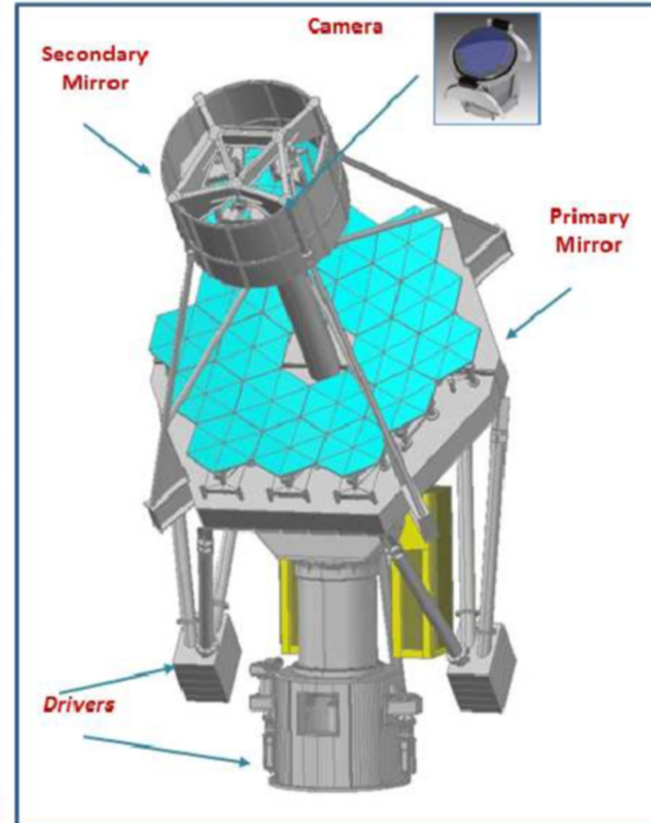
The primary mirror of the telescope has a 4.2 m diameter
