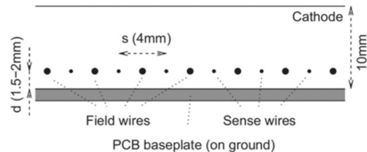
Fig. 3. The inner structure of a Close Cathode Chamber [10].
