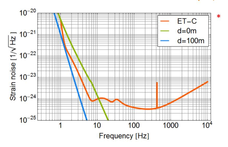
Infrasound NN in low frequency detectors for GW and earthquakes (TOBA, TORPEDO, atom interferometers)
