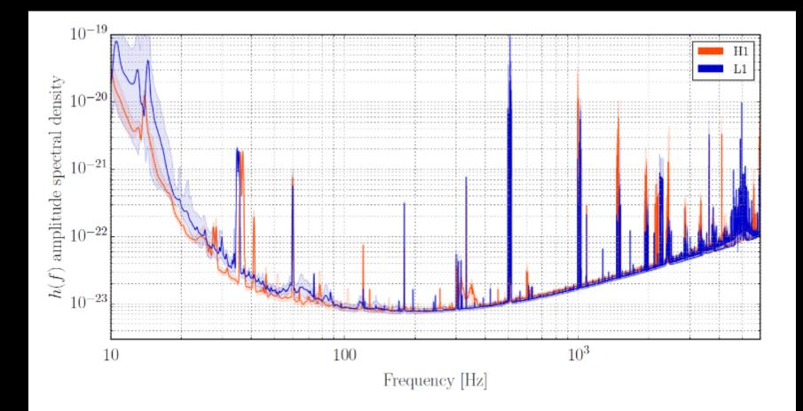
average measured strain-equivalent noise, of the Advanced LIGO detectors during Sept 12 - Oct 20, 2015
