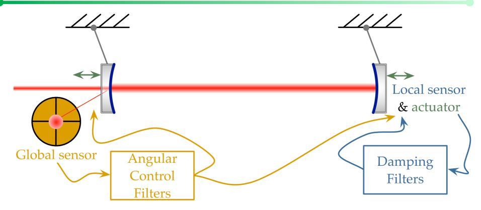
Can we use the local damping to smooth the Sigg-Sidles resonances so that we don't need to change global control filters as a function of laser power?
