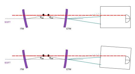
Locking the bench to the mirror might actually work, just amplifies the error signal for soft mode alignment
