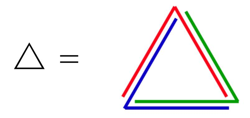
Might be confusing: current ET design has two interferometers per detectors (xylophone). But those could be replaced by **one** Michelson/speedmeter/... each. This is **not relevant** for the discussion of the triangle as a detector shape.
