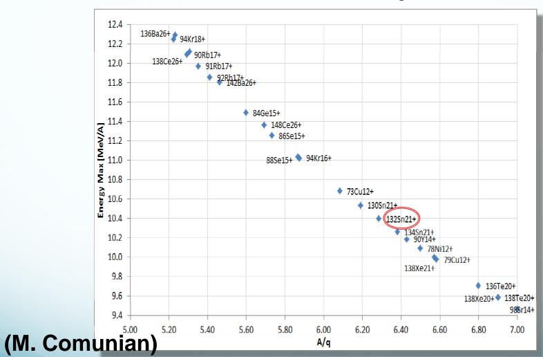
Preliminary results from alpi performances with 2 cavities as margin, Low Beta=5 MV/m, Medium Beta=4.3 MV/m, High Beta=5.5 MV/m Giacomo de Angelis
