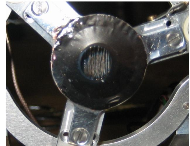
→ modified target to increase heat conductivity:
