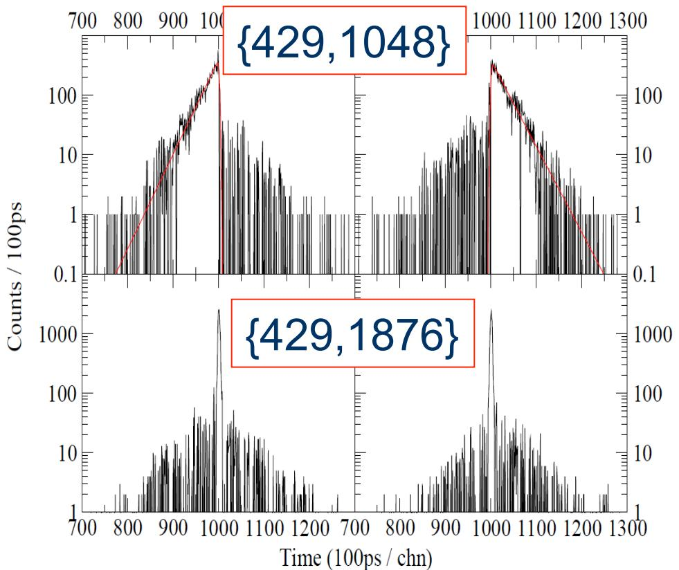
$T_{1/2}(4^-) = 2.0(2)$  ns ;  $4^- \rightarrow 2^+$  = M2 decay. Consistent with ‘pure’  $\pi f_{7/2} \rightarrow \pi d_{3/2}$  transition.
