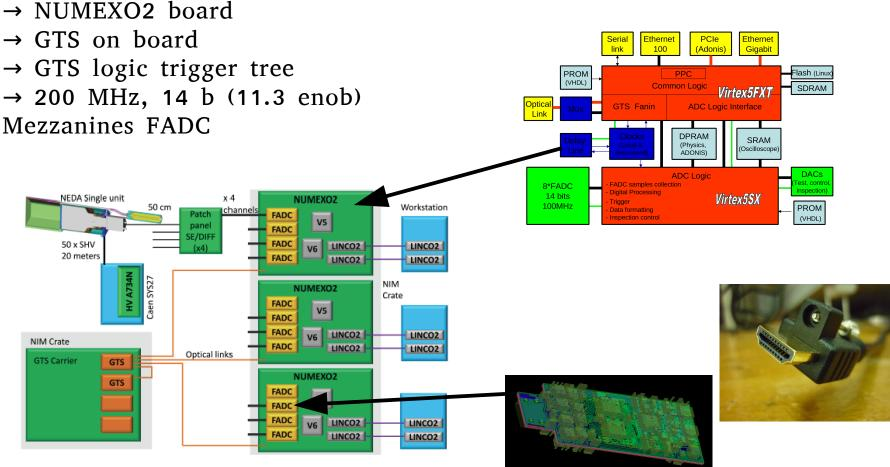
Figure 20: Global electronics layout for 48 NEDA detectors
