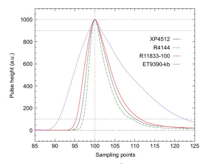
**Fig. 2.** Digitized waveforms averaged over 10<sup>5</sup> events for the four 5 in. PMTs coupled to a cylindrical 5 in. by 5 in. BC501A. The sampling frequency of the digitizer was 500 MS/s. The waveforms were normalized to a pulse height of 1000 and time aligned at the maximum of the signal. Dashed lines are drawn at 10%, 90%, at the maximum and at the baseline of the waveform to guide the eye.
