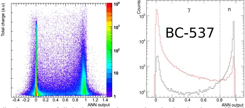
Full advantage of digital electronics can be obtained using artificial neural networks to perform pulse-shape discrimination. This method is currently being investigated both for BC537 and BC501A.
