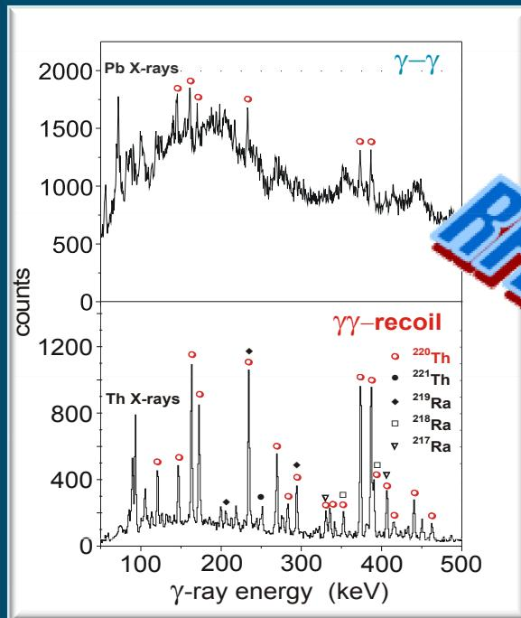
$68 \text{ MeV}^{18}\text{O} + 0.8 \text{ mg/cm}^2 {}^{30}\text{Si}$
