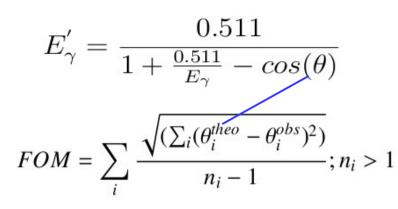
FOM : a measure of how well the interaction angles and interaction energies follow the Compton scattering formula inside a gamma ray
