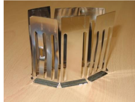
A melted RF finger (SOLEIL)
