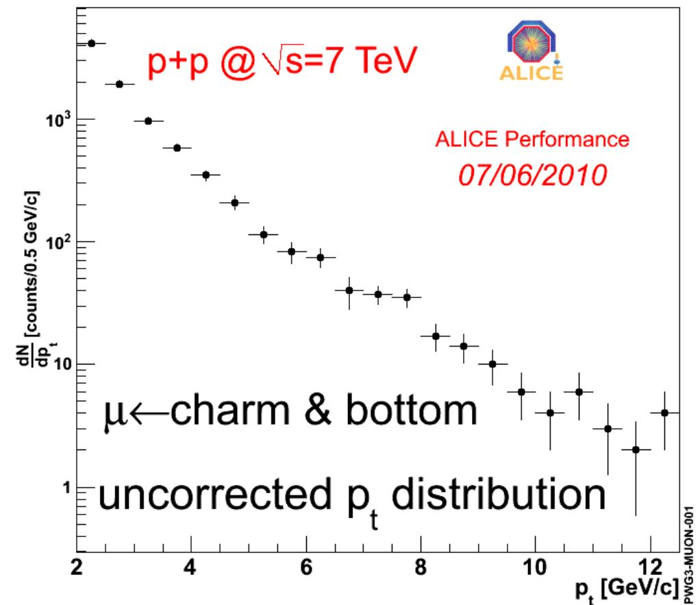
trigger chamber matching removes background (leads to cleaner Distance-of-Closest-Approach) ...remainder subtracted based on Pythia
