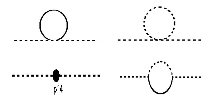
Dotted line: pion propagator , Solid line: scalar propagator
