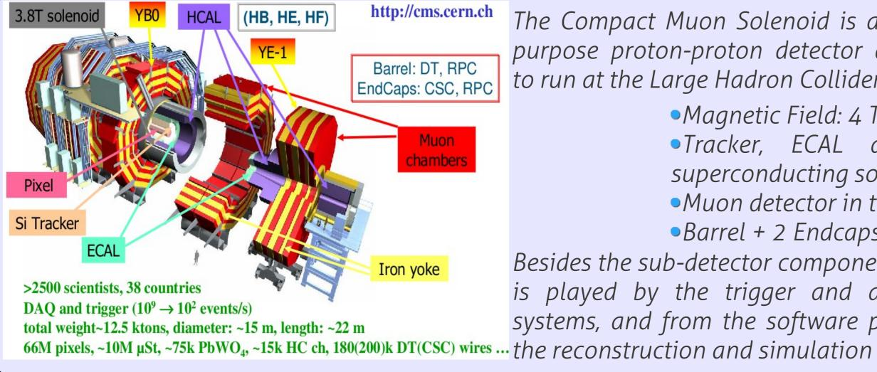
The Compact Muon Solenoid is a general purpose proton-proton detector designed to run at the Large Hadron Collider •*Magnetic Field: 4 T (3.8 T at the start-up)*
