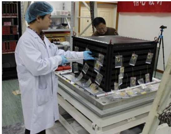
BGO crystal installation
