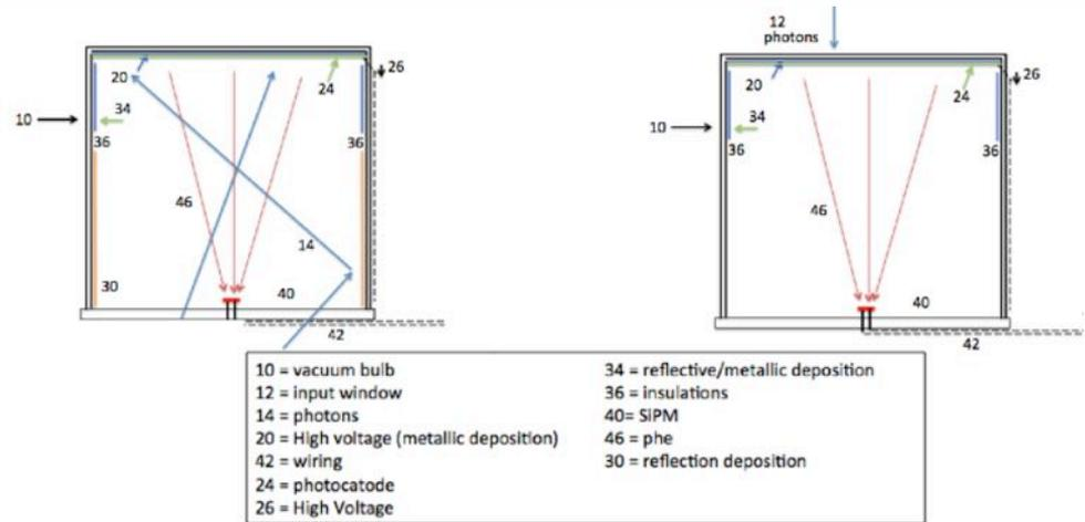
A new configuration for an higher QE in the VUV
