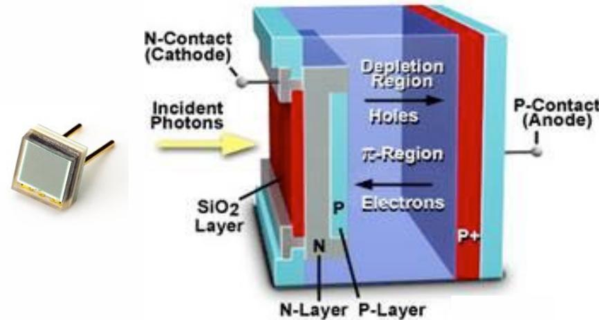
**PARALLEL GAIN:** obtained with the Geiger-avalanche generated in the p-n junction
