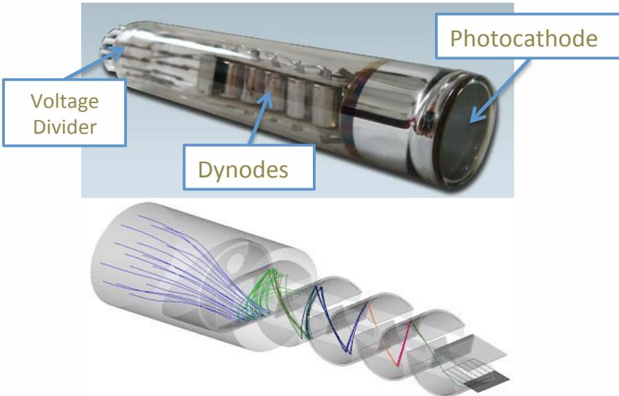
**SERIAL GAIN:** obtained by multiplying the photoelectrons in the dynodes
