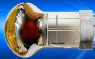
The classical dynode chain of a PMT is replaced with a special windowless p-over-n SiPM, acting as an electron multiplier (e-SiPM).
