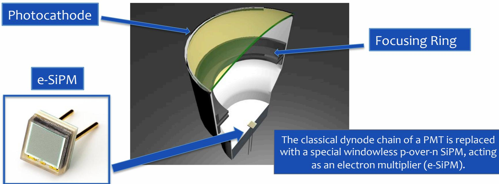
An innovative design for a modern hybrid photodetector based on the combination of a Silicon PhotoMultiplier (SiPM) with a hemispherical vacuum glass PMT standard envelope
