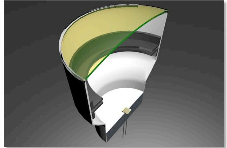
Thanks to the digital output of the e-SiPM the resolution of the whole device will be improved with respect to a classical PMT
