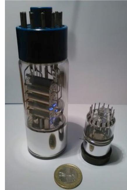
The VSIPMT is more compact and simpler having **ONLY 3 OUTPUT CONNECTIONS**: HV, SiPM bias voltage and the output signal.
