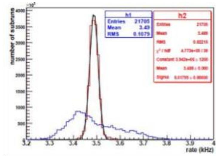
Intrinsic Trigger Rate stability 0.5% (after corrections for T/p effects)
