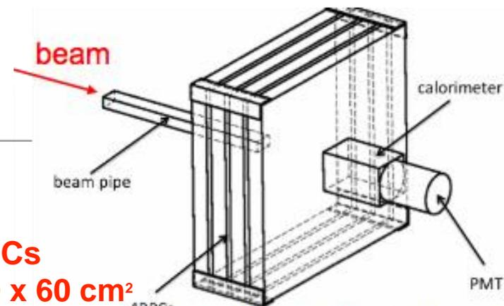
Calorimeter: lead glass block from OPAL, PMT a Hamamatsu R2238.
