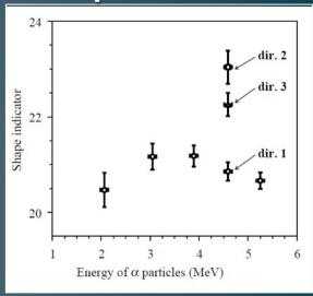
These anisotropic effects are ascribed to preferred directions of the excitons' propagation in the crystal lattice affecting the dynamics of the scintillation mechanism
