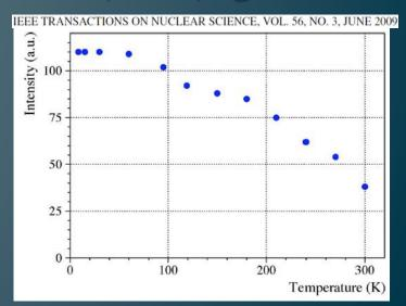
Light output measured for a ZnWO4 scintillator with  $^{241}$ Am  $\alpha$  particles as function of Temperature
