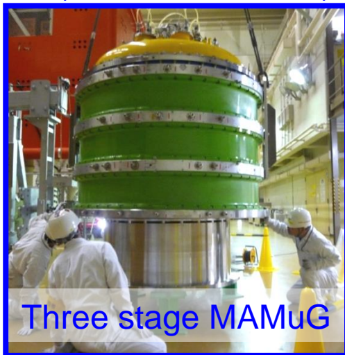
Accelerator of JT-60U NBI (500 keV, 22 A, D - )
