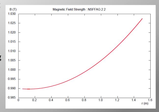
Magnet geometry optimised with field gradient to create isochronous machine
