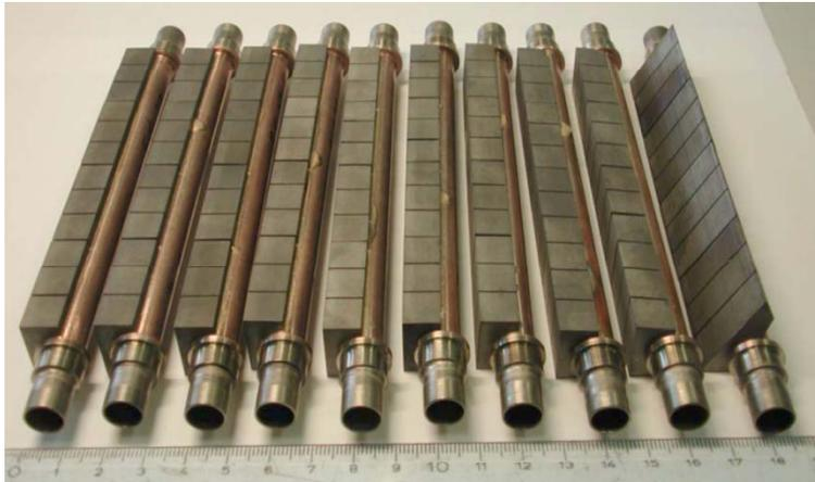
1. Be-tile brazed cooling pipes with Zr adapters
