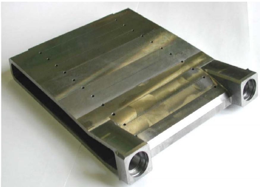
1. Target shaping from solid Be block machining
