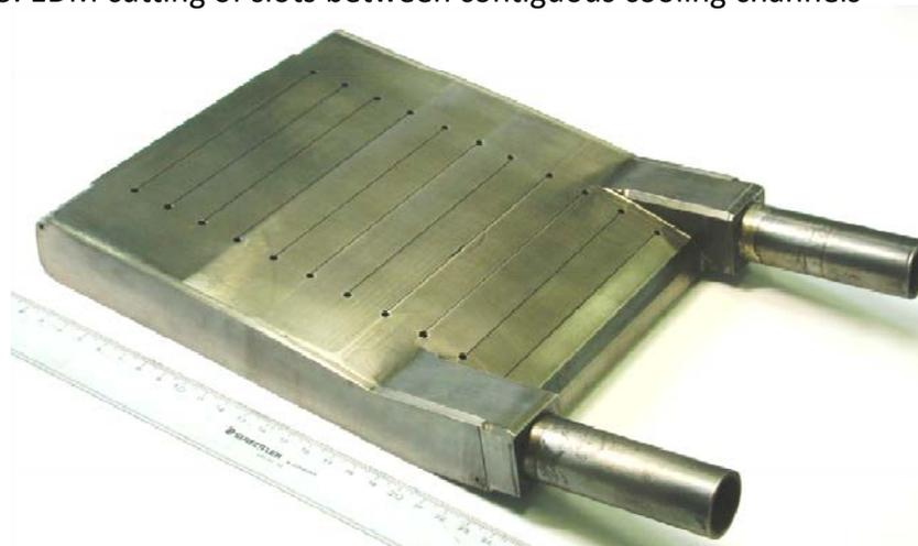
4. Half target after cover plates + joining pipes brazing
