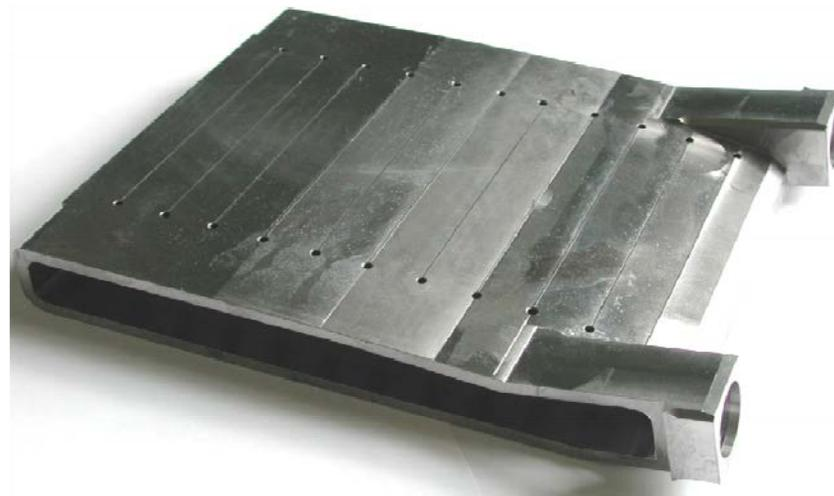
3. EDM cutting of slots between contiguous cooling channels
