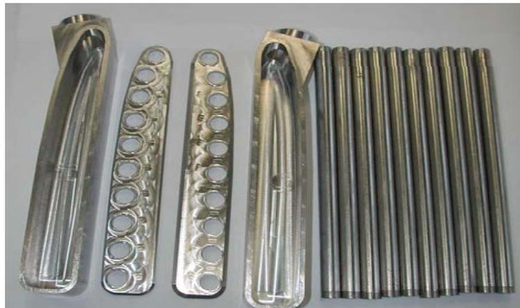
2. Zr cooling system manifold & collector plates
