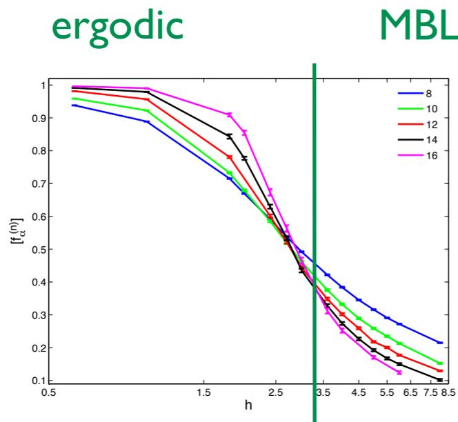
FIG. 2: (Color online) The fraction of the initial spin polarization that is dynamic (see text). The sample size  $L$  is indicated in the legend. In the ergodic phase (small  $h$ ) the polarization decays substantially under the dynamics, while in the localized phase (large  $h$ ) the decay is small, and this distinction gets sharper as  $L$  increases.
