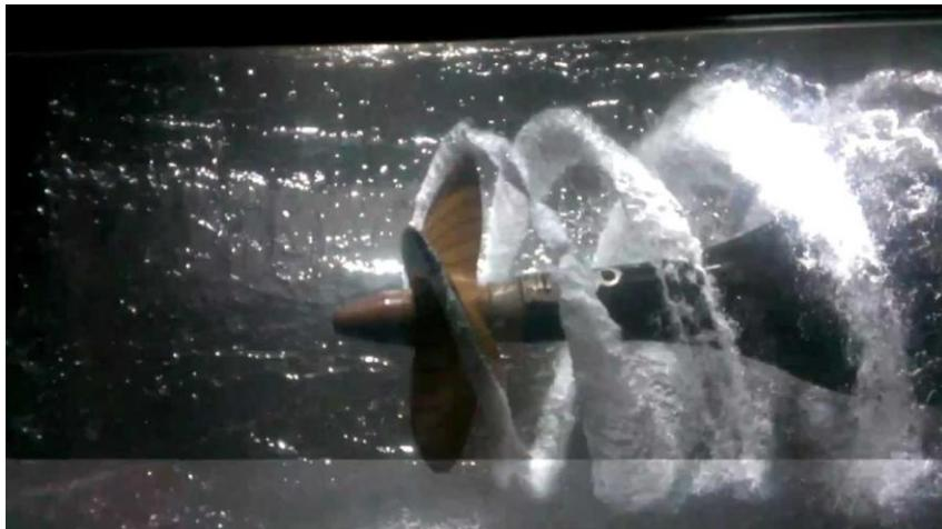
Cavitation on ship propellers
