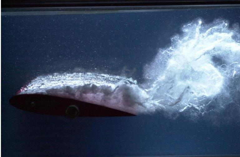
*Cavitation behind a NACA 0015 hydrofoil<sup>2</sup>*
