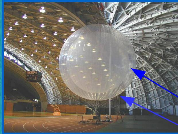
Two Nylon balloons 150  $\mu\text{m}$  thick
