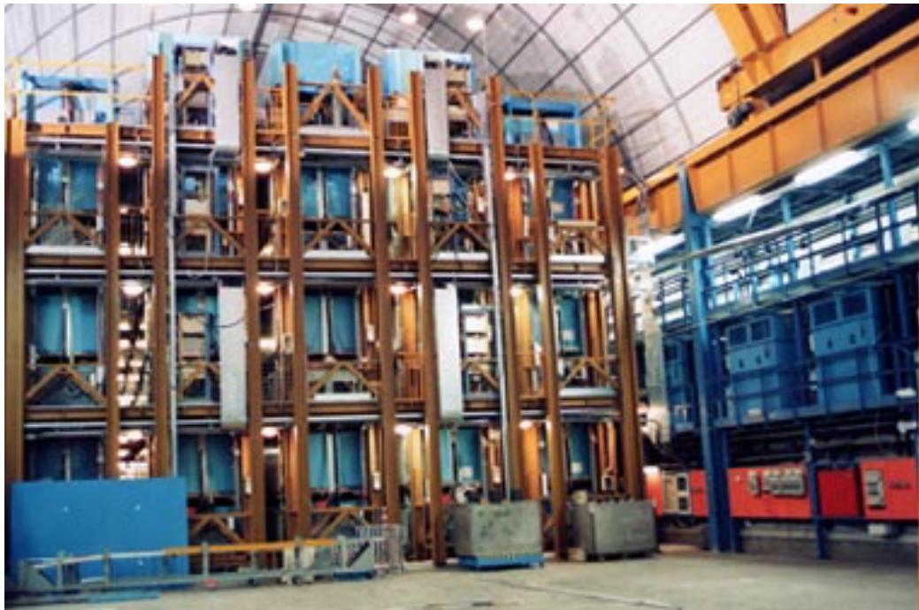
LVD consists of an array of 840 scintillator counters, interleaved by streamer tubes, and arranged in a compact and modular geometry.
