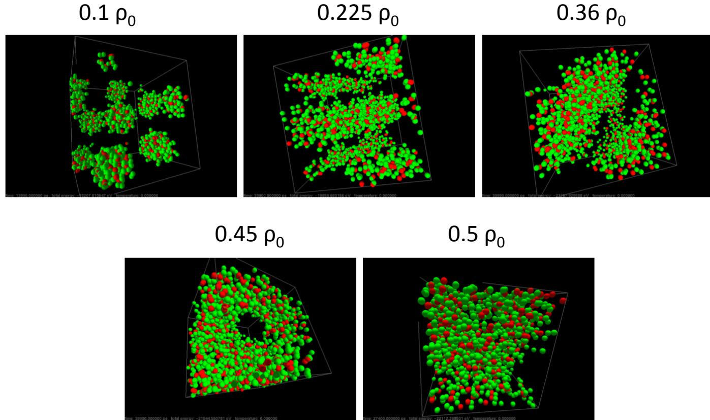
structures for different densities at fixed proton to neutron ratio  $Y_p = 0.31$
