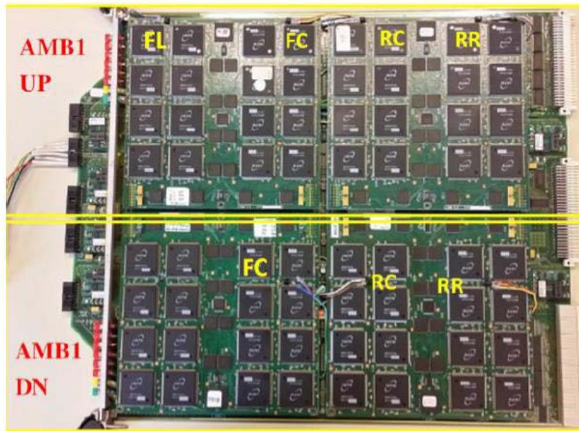
Positions of the 12 T sensors on an AMBSlim. Only three AMBSlim were equipped with sensors
