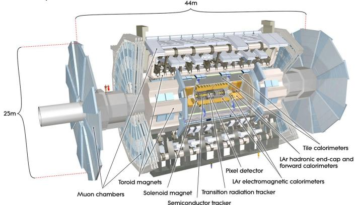
After a 3-year data taking phase (Run-I, 2010-2012) and a 2-year shutdown (LS1, 2013-2014) for repairing and upgrade, the ATLAS Detector is again operational at the LHC Run-II at √s=13TeV
