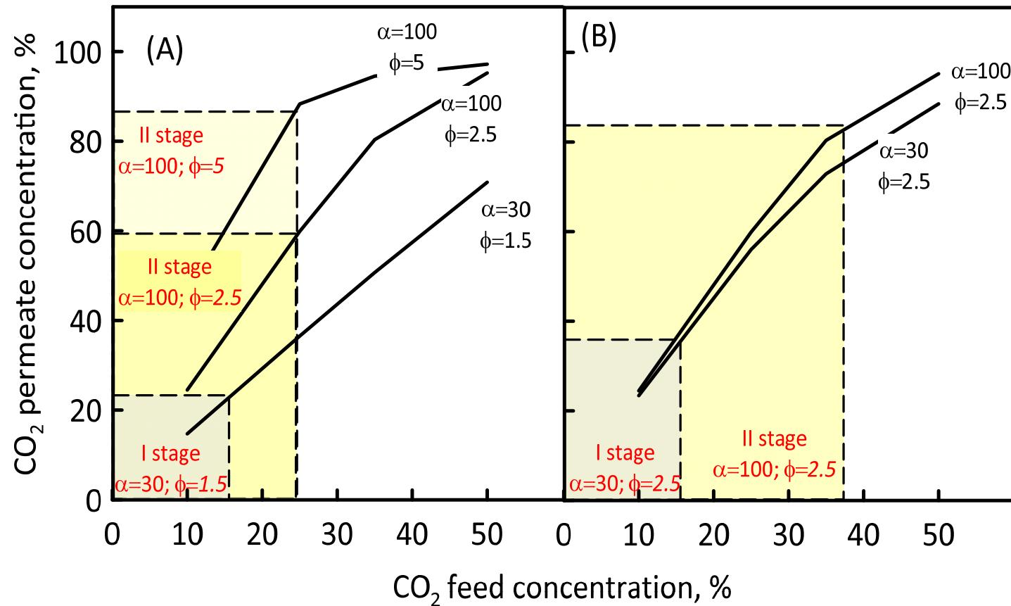
$\text{CO}_2$  permeate concentration as function of  $\text{CO}_2$  feed concentration at different selectivities for a multistage configuration
