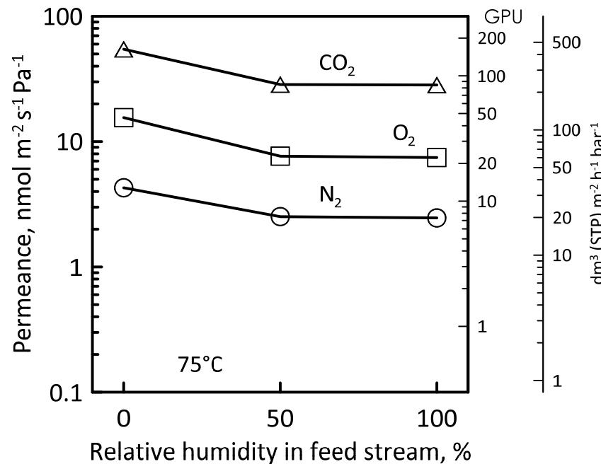
As the feed gas becomes increasingly humidified, the corresponding CO<sub>2</sub>, N<sub>2</sub> and O<sub>2</sub> permeance decreases. This permeance fall is owing to a competitive sorption and also declining diffusivities owing to blockage by water clusters at a higher relative humidity [Colin A. Scholes, Benny D. Freeman, Sandra E. Kentish, journal membrane science 470 (2014) 132-137].
